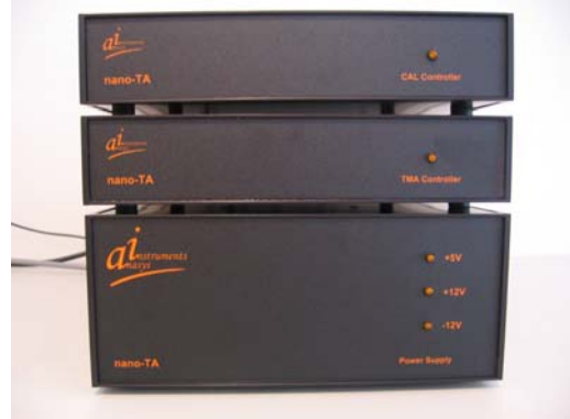
The nano-TA electronics comprising the power supply, TMA controller and CAL box.
